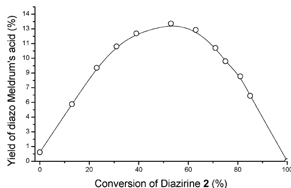
Figure 10. Formation of diazo Meldrum's acid ( 1 ) in 300 nm photolysis of diazirine 2 in methanol.
